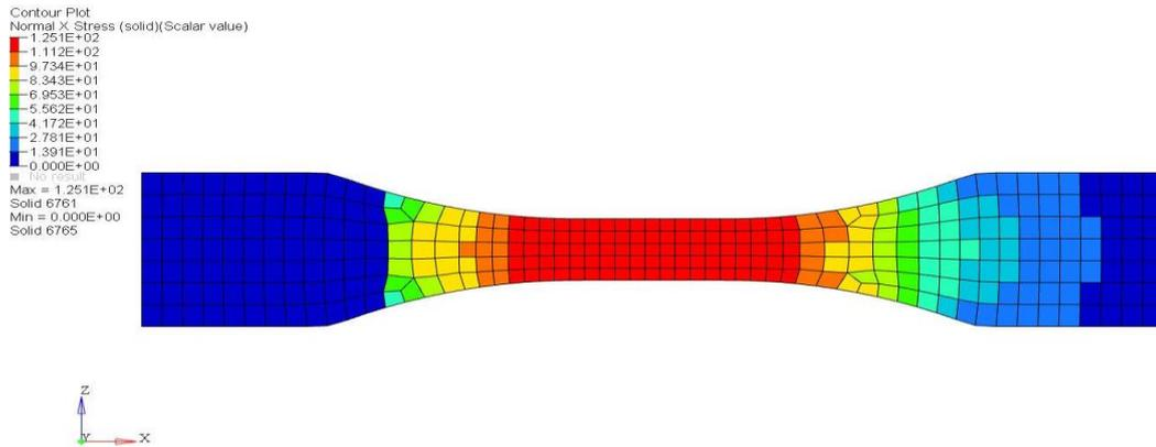
Figure 5: Finite element result of the miniature specimen to check the stress contraction.
