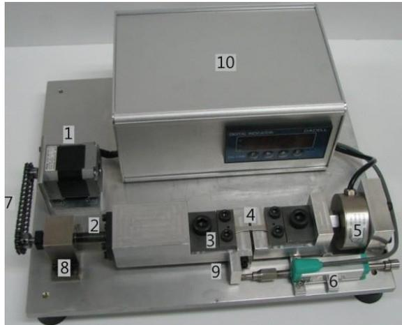
Figure 1 shows the overall structure of the miniaturised tensile testing machine.
