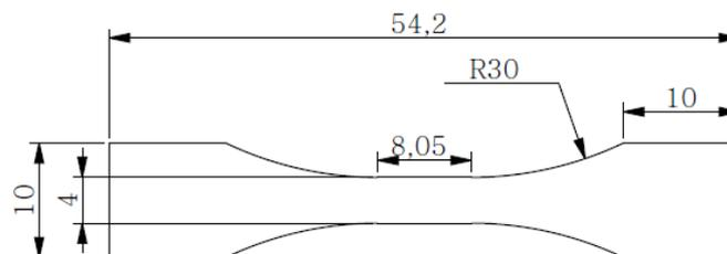
Figure 4: Dimensions of the miniature tensile specimen.
