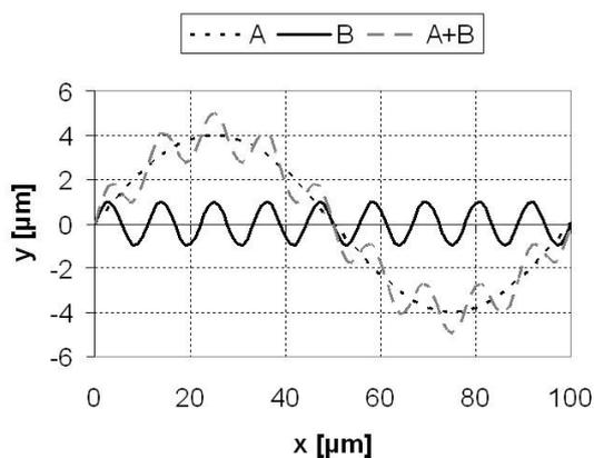
**Fig. 1.** Rough surface modeled as two-scale surface. In case of “smooth” surface, there are no fine scale asperities on top of the coarse scale asperity.
