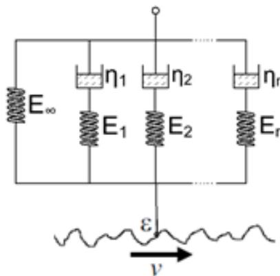
**Fig. 2.** Model for the computation of viscoelastic friction.
