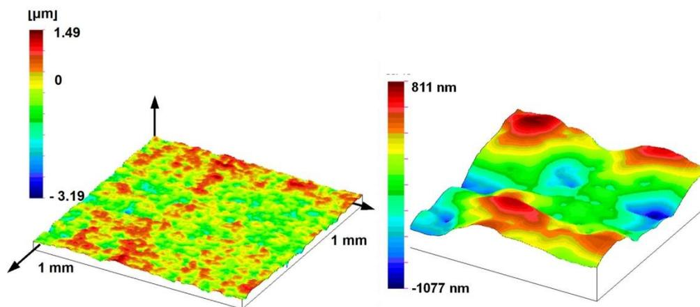
Fig. 2. Topographies measured by stylus (left) and measured by AFM (right)
