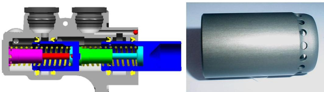
**Fig. 1.** Scheme of brake system (left) and the measured primary plunger (right)
