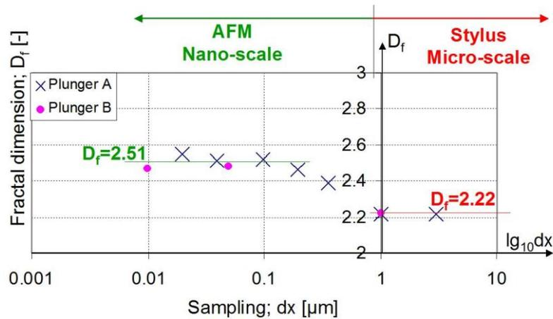
Fig. 3. Fractal dimensions of the plunger in different scales
