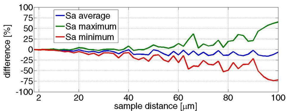
Fig. 2. The minimum, maximum and average Sa values in a function of sample distance
