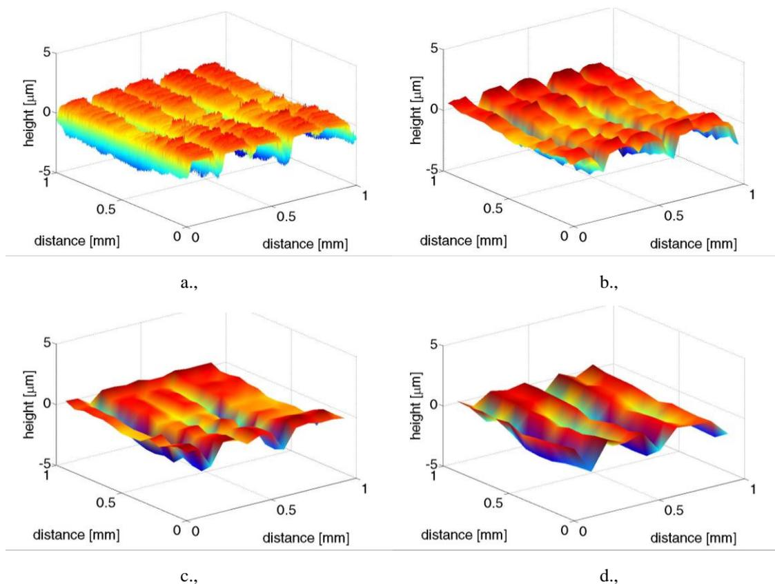
**Fig. 1.** Use 'The original (a) and the simulated microtopography with 34 micron (b), 68 micron (c) and 100 micron (d) sample distance.
