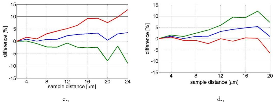
**Fig. 3.** The minimum, maximum and average Sa (a) Sq (b) Ssk (c) and Sku (d) values in a function of sample distance
